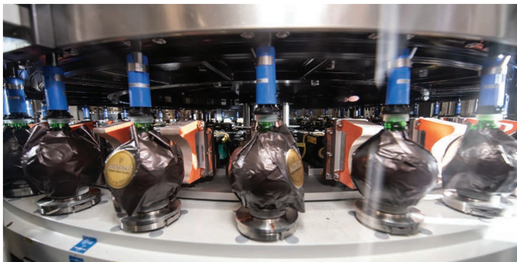
Patented solution for affixing the foil: a servomotor turns the bottles, while linear motors press the foil onto the containers with the aid of sponges
